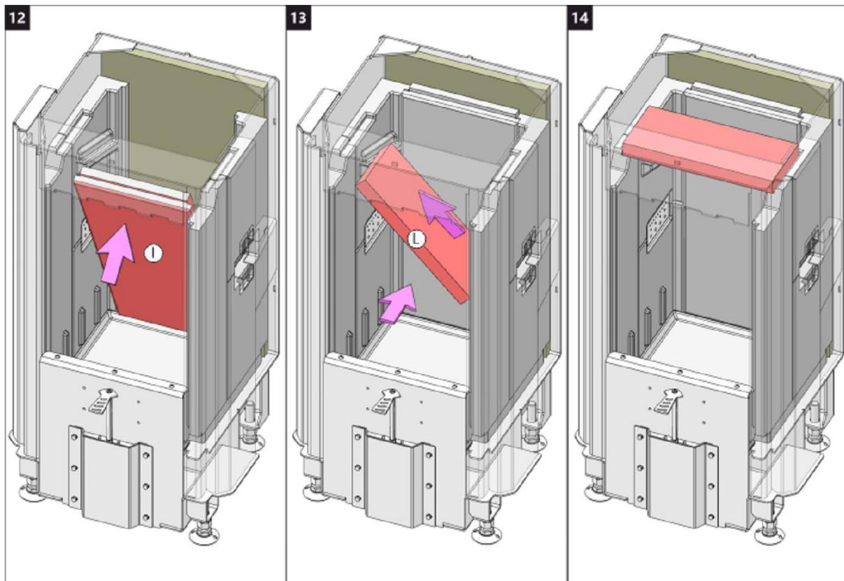
**Burning chamber 7 | Brennkammer 7 | Chambre de combustion 7 | Camera di combustione 7**
