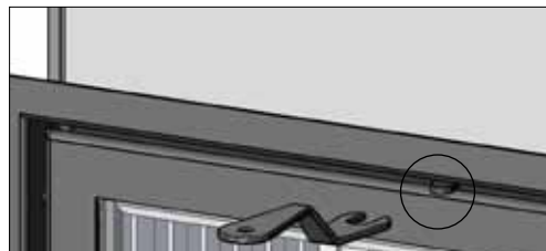
Ignition vent / Air vent control
